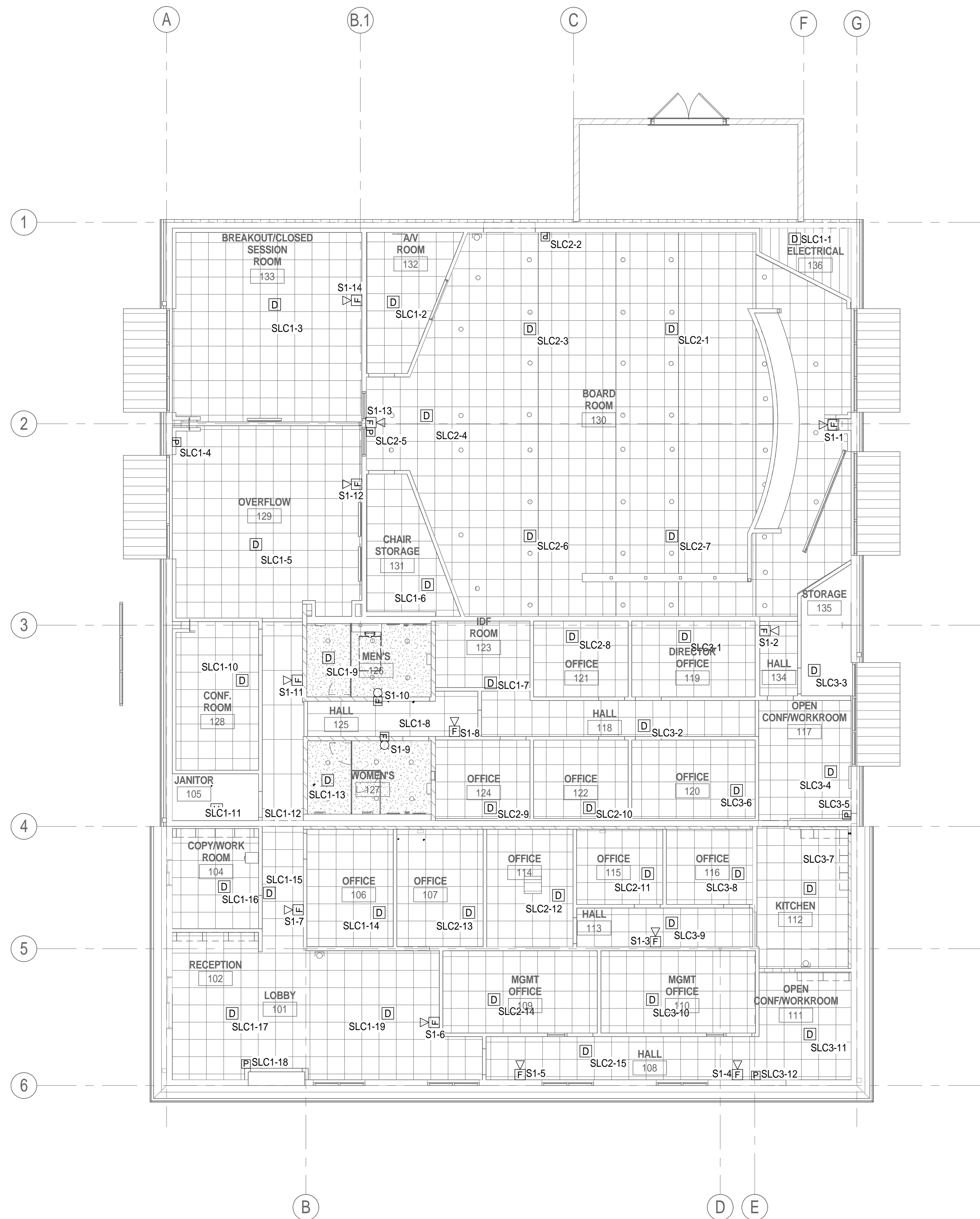
1 FIRE ALARM PLAN 1/8" = 1'-0"
